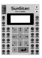
B. Press No. 5 key for threading. The following message is displayed on the screen, and all keys become disabled. The sewing operation pedal switch is also disabled.
