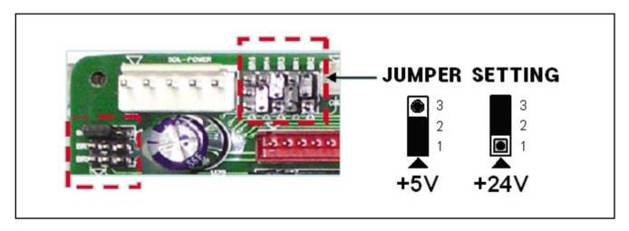
▶ The input power supply to the sensor can be altered to +5V / +24V by changing the BR jumper at the upper left side of the I/O board.
