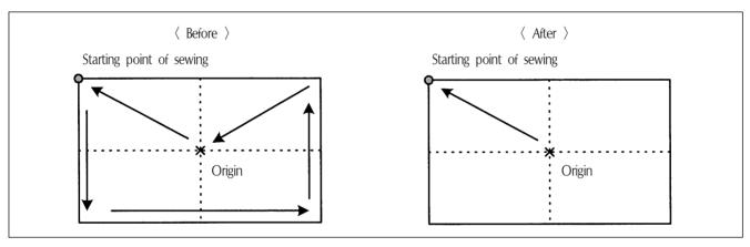
As SPS-1811 machines is equipped with reverse devices, origin search motion is performed as shown in the Before picture and feeds back to the starting point of sewing. However, if there is no reverse device, search motion takes place very slowly. This quick origin search motion function ensures fast origin search as shown in the After picture and feeding back to the starting point of sewing.
