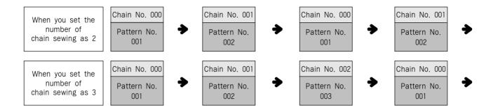
It is used to work with the various patterns randomly. To use the function, the parameter number related to general sewing, "054 Chain No." should be set to the other numbers except "0". Set the parameter number related to general sewing, "055 Chain Select." to be automatic or manual.
